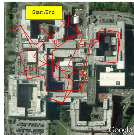
Figure 4: IMU+ ZUPT solution
