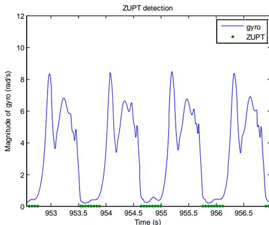
Figure 2. Exampe of ZUPT detection using angular rates detection
