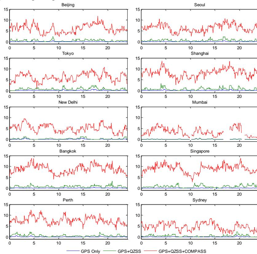
Figure 9: “Nines” of the single-frequency ambiguity resolution success rate for different combination at selected cities (above a 30 degree cutoff angle).
