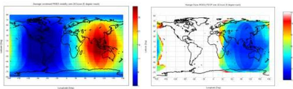
Figure 7: Average number of visible satellites (left) and average PDOP value (right) of combined RNSSs over a 24 hour period (above a five degree elevation cutoff angle)
