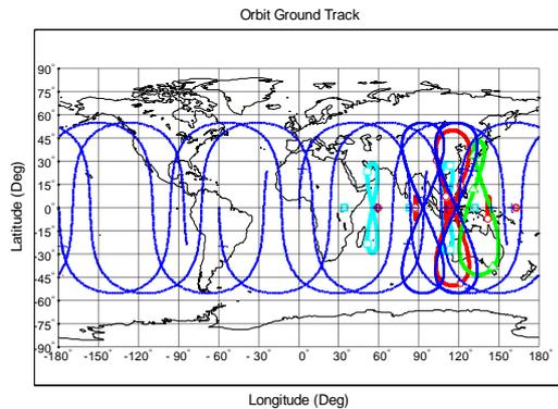
Figure 1: The satellite ground tracks of IRNSS (in cyan with squares), Compass phase II (in blue with crosses), QZSS (in green with triangles) and CAPS (in red with circles).
