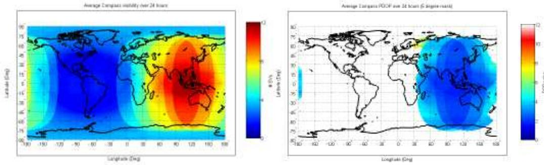
Figure 5: Average number of visible satellites (left) and average PDOP value (right) of the Compass phase II constellation over a 24 hour period (above a five degree elevation cutoff angle)
