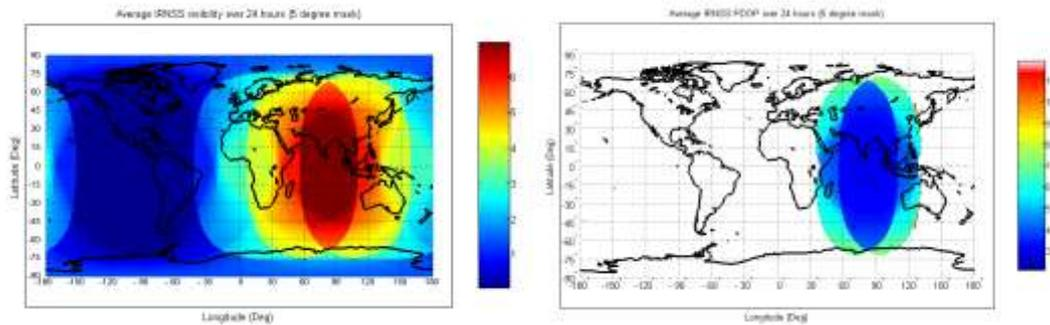
Figure 3: Average number of visible satellites (left) and average PDOP value (right) of the IRNSS constellation over a 24 hour period (above a five degree elevation cutoff angle) – white area indicates that the PDOP value is higher than 12
