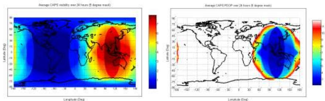
Figure 4: Average number of visible satellites (left) and average PDOP value (right) of the CAPS constellation over a 24 hour period (above a five degree elevation cutoff angle) – white area indicates that the PDOP value is higher than 12
