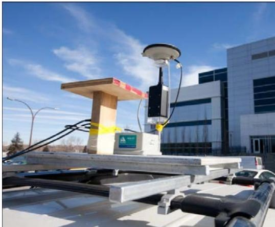
Figure 2: GPS, UWB and IMU Equipment Setup on a Test Vehicle
