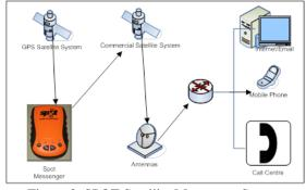
Figure 3: SPOT Satellite Messenger System
