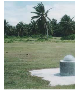
Fig. 8 COCO station is equipped with an ASHTECH UZ-12 GPS receiver with an AOAD/M_T antenna type. This station is located within the perimeter of Cocos Island Airport and it offers unobstructed visibility of the sky (Geoscience Australia, 2007).
