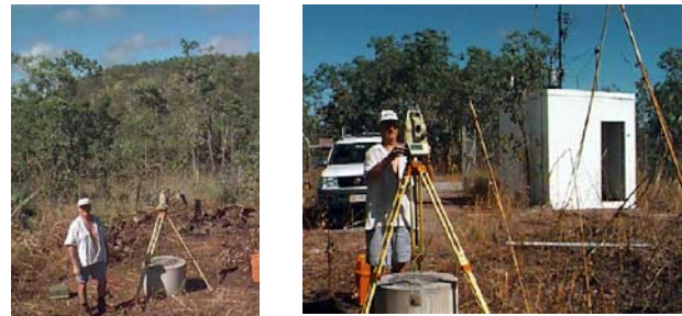
Fig. 9 DARW station is equipped with an ASHTECH UZ-12 GPS receiver with an ASH700936D_M antenna type. This station is located at an old abandoned seismic station at Manton Dam and is surrounded by trees and a building (Geoscience Australia, 2007).
