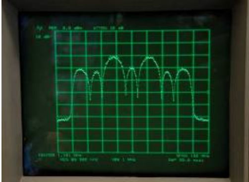
Fig. 5 PSL RF Transmitter Output Spectrum
