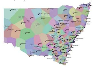
Fig. 2 Voronoi polygons of the assumed NSW network
