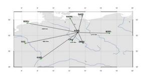
Fig. 3 Illustration of the real-time stations used in the experiment and the lengths of the baselines from the used reference stations to experiment kinematic stations in Potsdam, where POTS stands for A17B and A17D
