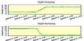
Fig. 6 Coordinate changes of station A17D in details during the height increasing and decreasing period, where the black lines represent the real track of the manual height changes and green dots are the real-time estimated coordinate changes compared to the true
