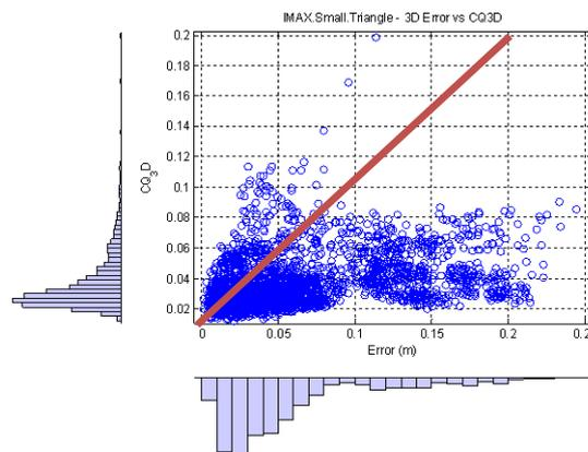
Figure 5: Illustration of 3D position errors plotted against 3D CQ indicator for i-MAX solution from a standard triangle network
