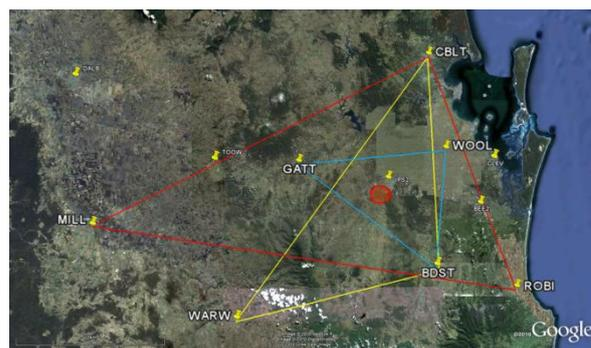
Figure 1: Combined SunPOZ and the CRCSI test network in SEQ with 3 test triangle networks
