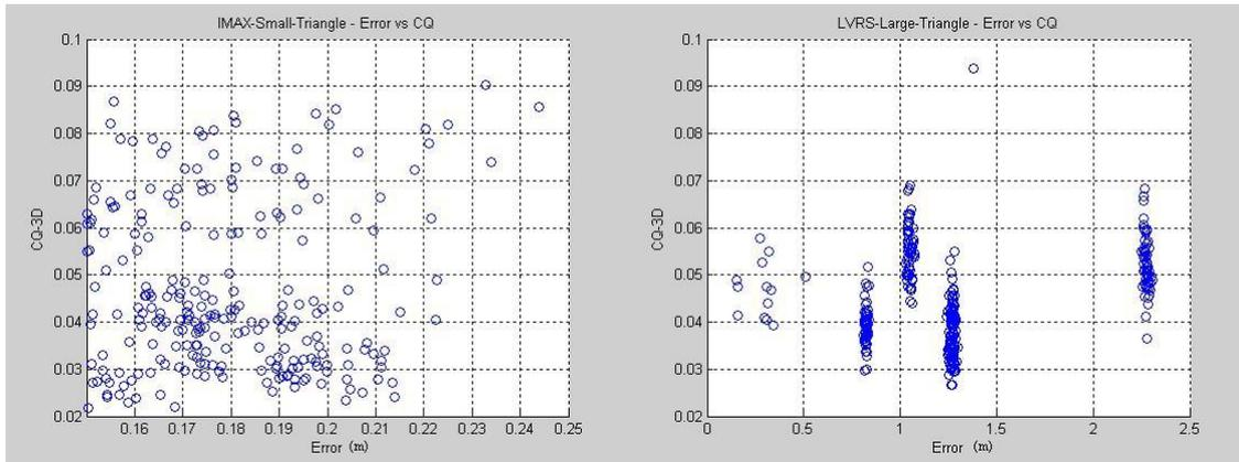
Figure 7: 3D error verse 3D CQ for Leica SmartNet i-Max solution (left) and VRS solution (right)
