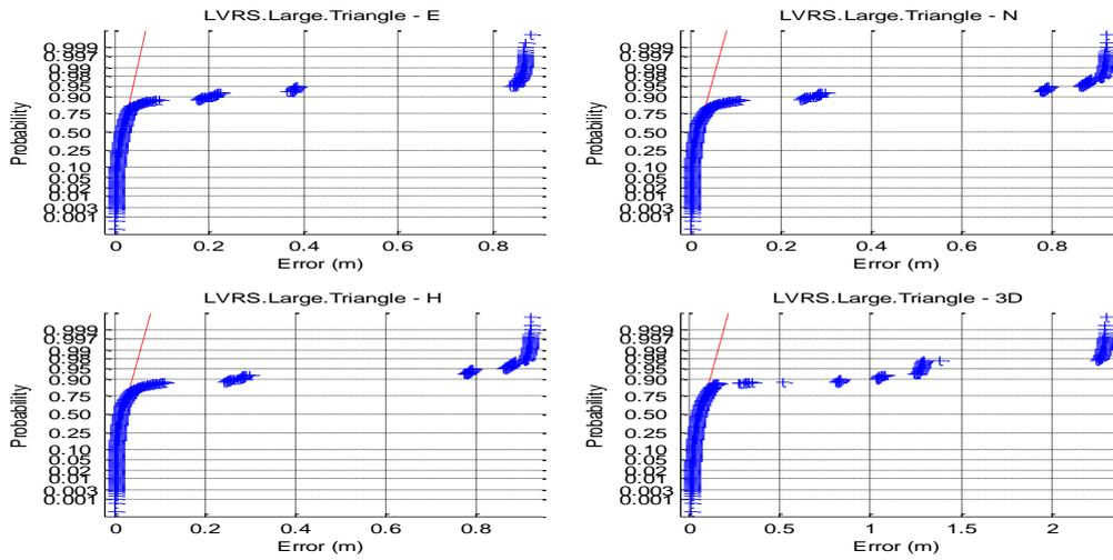
Figure 3: Accuracy of Leica SmartNet VRS solutions for large triangle network
