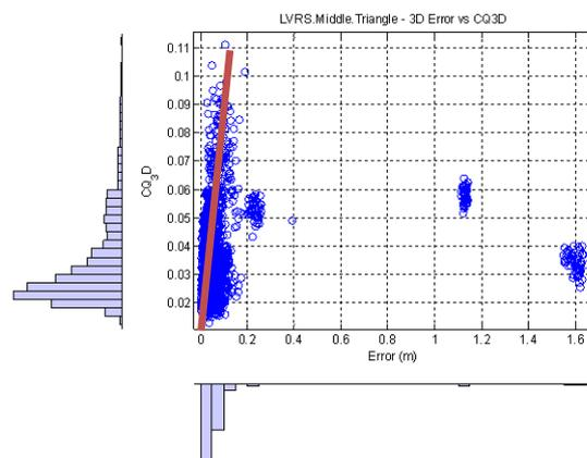
Figure 6: Illustration of 3D position errors plotted against the 3D CQ indicator for Leica SmartNet VRS solution from the large triangle network
