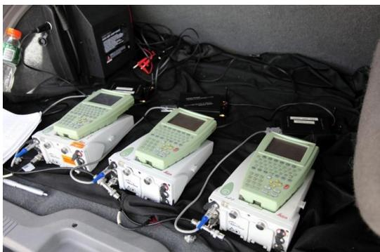
Figure 2: Leica Rovers used during the test. Each is connected with individual NextG modem and to a common GNSS antenna via the splitter.
