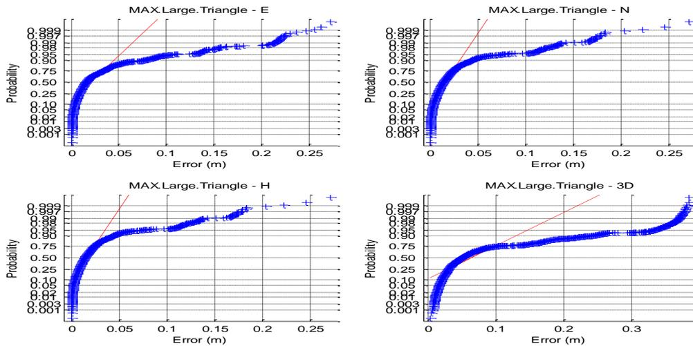
Figure 4: Accuracy of Leica SmartNet MAX solutions for large triangle network
