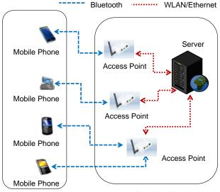
Figure 1: System components of the inquiry-based Bluetooth indoor locating system.
