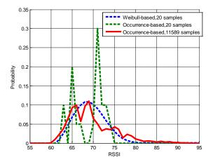
Figure 4: Weibull-based (k=2.5,  $\lambda$ =9.275,  $\theta$ =61) vs. occurrence-based probability distributions with 20 samples
