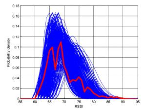
Figure 6: Probability densities estimated with Weibull functions for all sessions of 20 RSSI measurement samples. The red line is the benchmark distribution.
