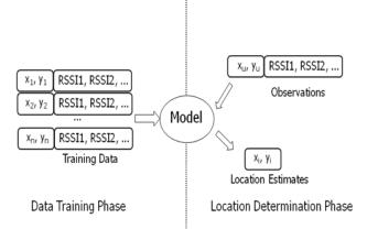
Figure 2: Two phases for Bluetooth positioning
