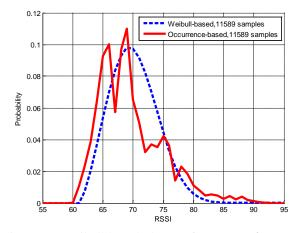
Figure 3: Weibull-based (k=2.5,  $\lambda$ =10.275,  $\theta$ =61) vs. occurrence-based probability distribution with 11589 samples
