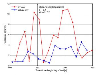
Figure 9: WLAN and Bluetooth locating errors
