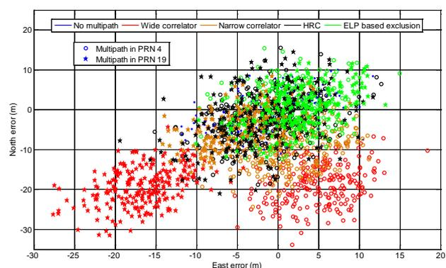
Figure 3: Positioning error on a two-dimensional plot for the scenarios considered in Fig. 2
