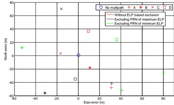
Figure 16: Positioning error for scenarios given in Table-I, when there are less than four multipath-free satellite signals available (latitude = 25°, longitude = 30°, UTC starting time = 1620 hrs on 15<sup>th</sup> November, 2009)
