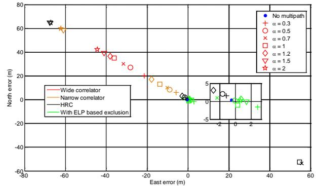
Figure 7: Mean positioning error for multipath in PRN 14 signal ( $d = 220$  m, latitude =  $-10^\circ$ , longitude =  $110^\circ$ , UTC starting time = 1510 hrs on 04<sup>th</sup> August, 2009) (inset: zoom of results around zero error)
