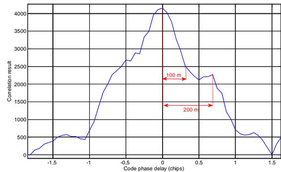
Figure 11: Correlation of a received signal with a local code in the presence of multiple reflections ( $d_1 = 100$  m,  $\alpha_1 = 0.5$ ,  $d_2 = 200$  m,  $\alpha_2 = 0.3$ ) as given in Fig. 9
