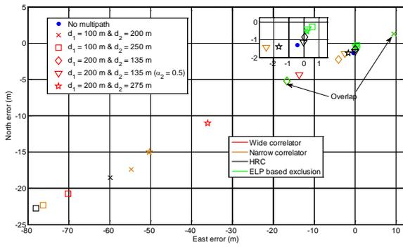
Figure 9: Mean positioning error for multiple reflections in PRN 11 signal ( $\alpha_1 = 0.5$ ,  $\alpha_2$  (unless stated otherwise) = 0.3, latitude =  $-20^\circ$ , longitude =  $-45^\circ$ , UTC starting time = 1500 hrs on 27<sup>th</sup> October, 2009) (inset: zoom of results around zero error)
