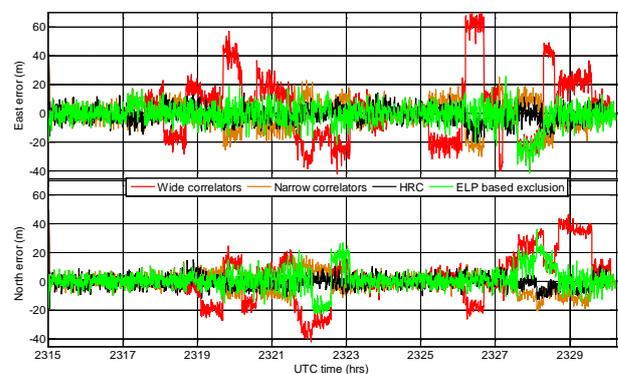
Figure 14: East and north error for multipath pattern given in Fig. 13
