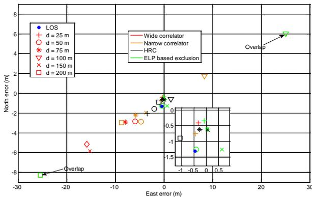
Figure 6: Mean positioning error for multipath in PRN 11 signal ( $\alpha = 0.5$ , latitude =  $-20^\circ$ , longitude =  $-45^\circ$ , UTC starting time = 1500 hrs on 27<sup>th</sup> October, 2009) Note the worst errors are not corrected using ELP-based satellite exclusion (inset: zoom of results around zero error).
