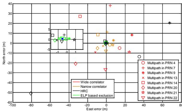
Figure 4: Mean positioning error for multipath in each individual satellite signal ( $\alpha = 0.5$ ,  $d = 220$  m, latitude =  $-10^\circ$ , longitude =  $110^\circ$ , UTC starting time = 1510 hrs on 04<sup>th</sup> August, 2009) (inset: zoom of results around zero error)
