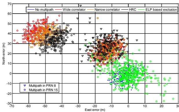
Figure 8: Positioning error due to the presence of dual reflections from the same satellite for latitude =  $-35^\circ$ , longitude =  $150^\circ$ , UTC starting time = 1020 hrs on 09<sup>th</sup> September, 2009 a) PRN 8 ( $\alpha_1 = 0.5$ ,  $d_1 = 255$  m &  $\alpha_2 = 0.7$ ,  $d_2 = 130$  m) b) PRN 15 ( $\alpha_1 = 0.5$ ,  $d_1 = 120$  m &  $\alpha_2 = 0.7$ ,  $d_2 = 65$  m)
