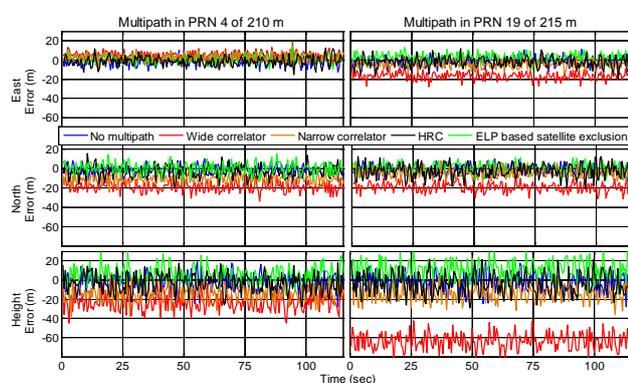
Figure 2: Positioning error due to multipath in a given constellation and effect of using ELP ( $\alpha = 0.5$ , latitude =  $-35^\circ$ , longitude =  $150^\circ$ , UTC starting time = 0708 hrs on 01<sup>st</sup> May, 2009)
