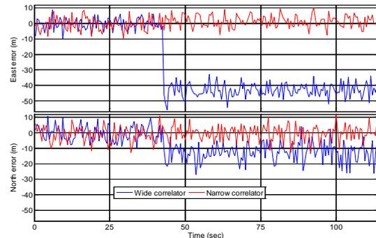
Figure 10: Positioning error for multiple reflections in PRN 11 signal as given in Fig. 9 but with first 40 seconds free of multipath ( $d_1 = 200$  m,  $\alpha_1 = 0.5$ ,  $d_2 = 275$  m,  $\alpha_2 = 0.3$ )
