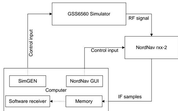
Figure 1: A block diagram of the experimental setup
