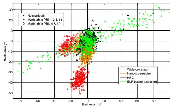
Figure 12: Positioning error due to the presence of dual reflections from two different satellites for latitude =  $-35^\circ$ , longitude =  $150^\circ$ , UTC starting time = 0708 hrs on 01<sup>st</sup> May, 2009 a) PRNs 12 & 18 ( $\alpha_{12} = 0.5$ ,  $d_{12} = 110$  m &  $\alpha_{18} = 0.5$ ,  $d_{18} = 85$  m) b) PRNs 4 & 19 ( $\alpha_4 = 0.5$ ,  $d_4 = 210$  m &  $\alpha_{19} = 0.5$ ,  $d_{19} = 215$  m)
