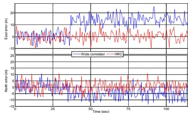
Figure 5: Positioning error for multiple in PRN 4 signal as given in Fig. 4 but with first 35 seconds free of multipath
