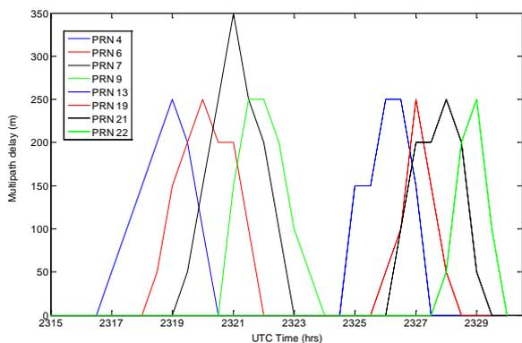
Figure 13: Path delay for multipath added over time for the experimental results of Fig. 14 and Fig. 15
