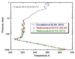
Fig. 3 GPS temperature profile compared with two radiosondes.
