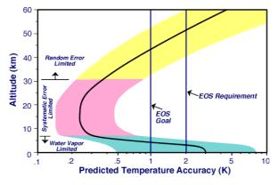
Fig. 2 Approximate occultation temperature accuracy vs altitude.
