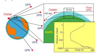
Fig. 1 Atmospheric temperature profiling by GPS occultation
