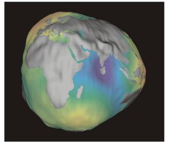
Fig. 2 Global gravity field model from three months of CHAMP data only
