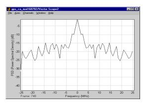
Fig.9 Unwanted signal/MAI signal level is 5dB larger than that of SOI
