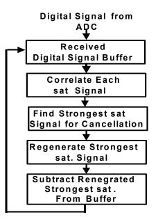
Fig. 6 Block Diagram of the Sequential Interference Cancellation (SIC)
