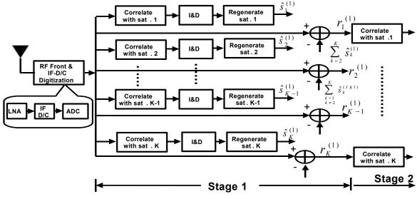
Fig 7. Block Diagram of Parallel Interference Cancellation
