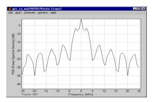
Fig 10 Unwanted signal/MAI signal level is 10dB larger than that of SOI
