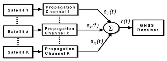
Fig. 1 GNSS CDMA channel model
