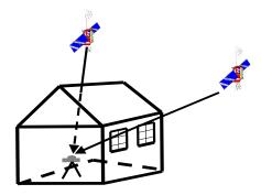
Fig. 4 Power level dispersion caused by different path attenuation
