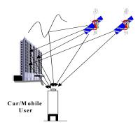
Fig. 5 Power level dispersion caused by multipath fading
