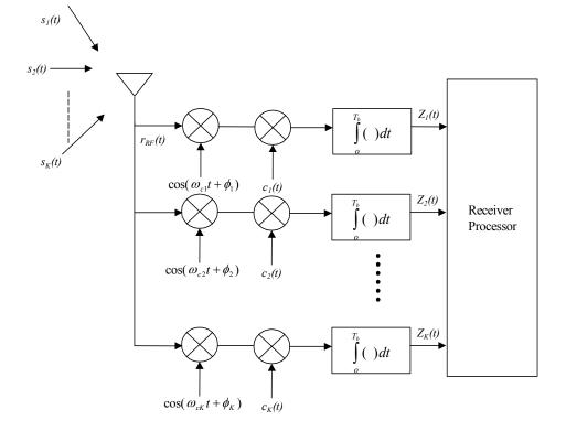
Fig. 2 A simplified bank of a conventional GNSS receiver structure for reception of the signals,  $s_1(t), s_2(t), ..., s_k(t)$ , from satellite 1, satellite 2, ..., satellite k, respectively
