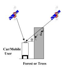
Fig. 3 Power level dispersion caused by tree attenuation
