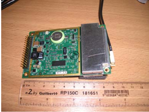
Figure 1 The JNS100 OEM board GPS receiver
