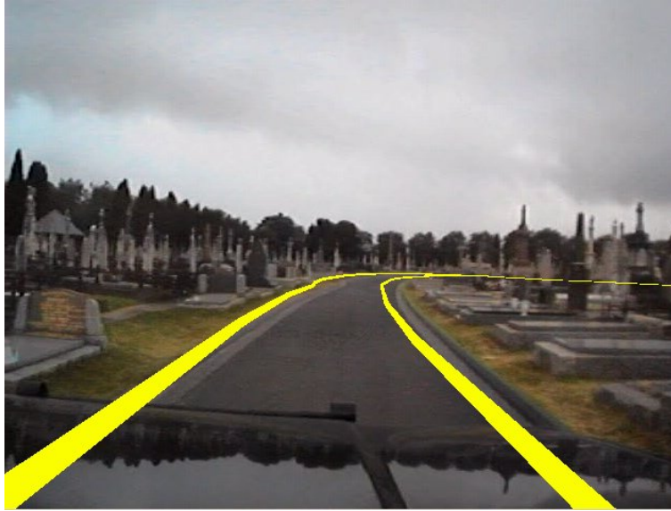
Figure 9 Misalignment of the augmented road boundaries caused by a 2 degree error in heading
