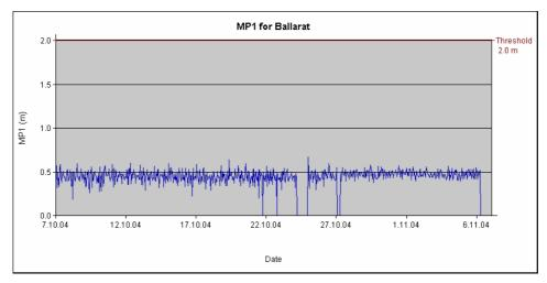
Fig. 3 Multipath effects detected for Ballarat station during October 2004
