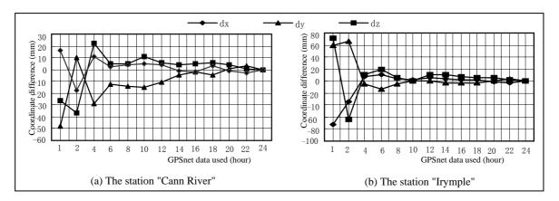
Fig. 8 Differences of the coordinate solutions in ITRF2000 using different session lengths of GPSnet data in comparison with the solution from 24 hours data
