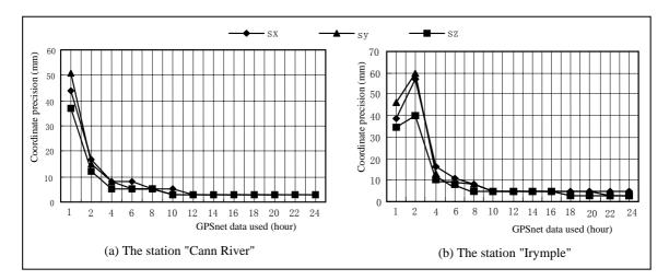
Fig. 7 Precision evaluation of GPSnet solution in ITRF2000 using different session lengths of data at stations (a) "Cann River" and (b) "Irymple" respectively
