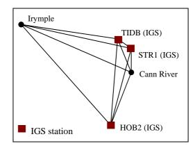
Fig. 6 An experimental network for precision analysis of GPSnet solution (not to scale)
