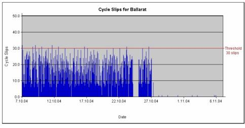
Fig. 2 Cycle slips detected for Ballarat station during October 2004
