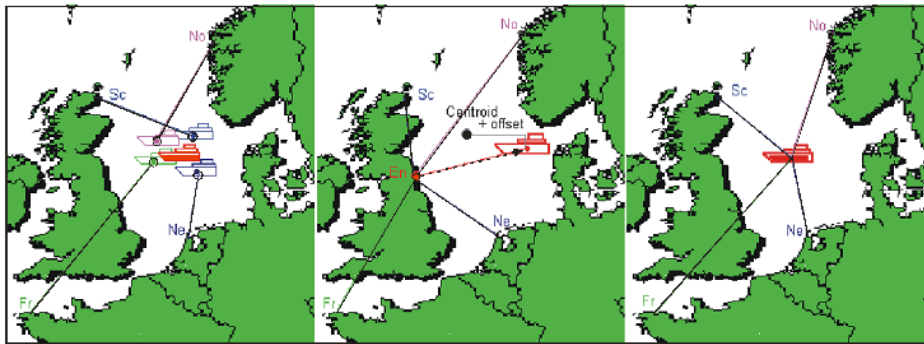
Fig. 3 The positioning methods using multi-DGPS references
