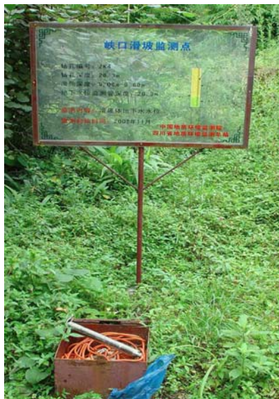
Fig. 6 Underground water level monitoring point
