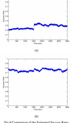
Fig 9 Comparison of the Estimated Success Rates (a:C/A Code Only, b:UKF+INS/GPS)
