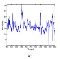
Fig. 3 Attitude determination result using C/A code and baseline constraint
