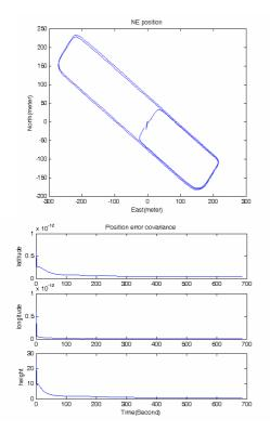
Fig. 5 Vehicle trajectory and the covariance of positioning result
