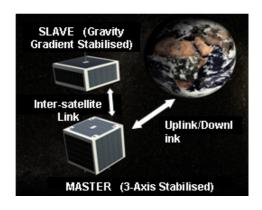
Fig 4 JAESat Communication Concept
