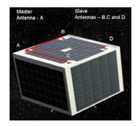
Fig 7 SPARx antenna array for JAESat 3-axis attitude determination. antenna D will be optional
