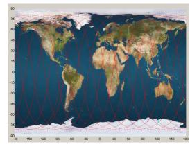
Fig 2 JAESat ground track
