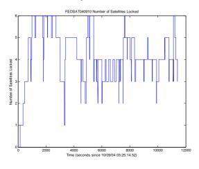
Fig 11 SPARx tracked GPS signals for a typical orbit scenario
