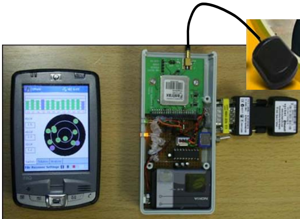
Fig. 7. User terminal of the EGNOS pseudolite system.
