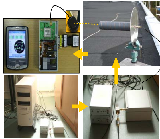
Fig. 8. Components of the EGNOS pseudolite system.
