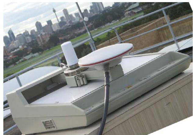
Fig. 5 HP XY plotter table with Locata and Leica AT502 antennas.
