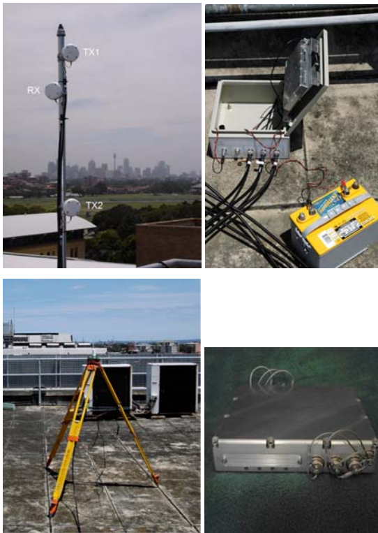
Fig. 2 LocataLite (5) antenna setup (top left) and weatherproof enclosure (top right). Locata receiver antenna setup (bottom left) and Locata receiver (bottom right).
